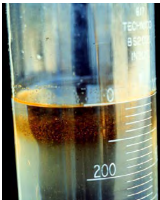
Figure 26. Layer of empty Striga seed coats floating on the potassium carbonate solution at the top of the separatory funnel.
