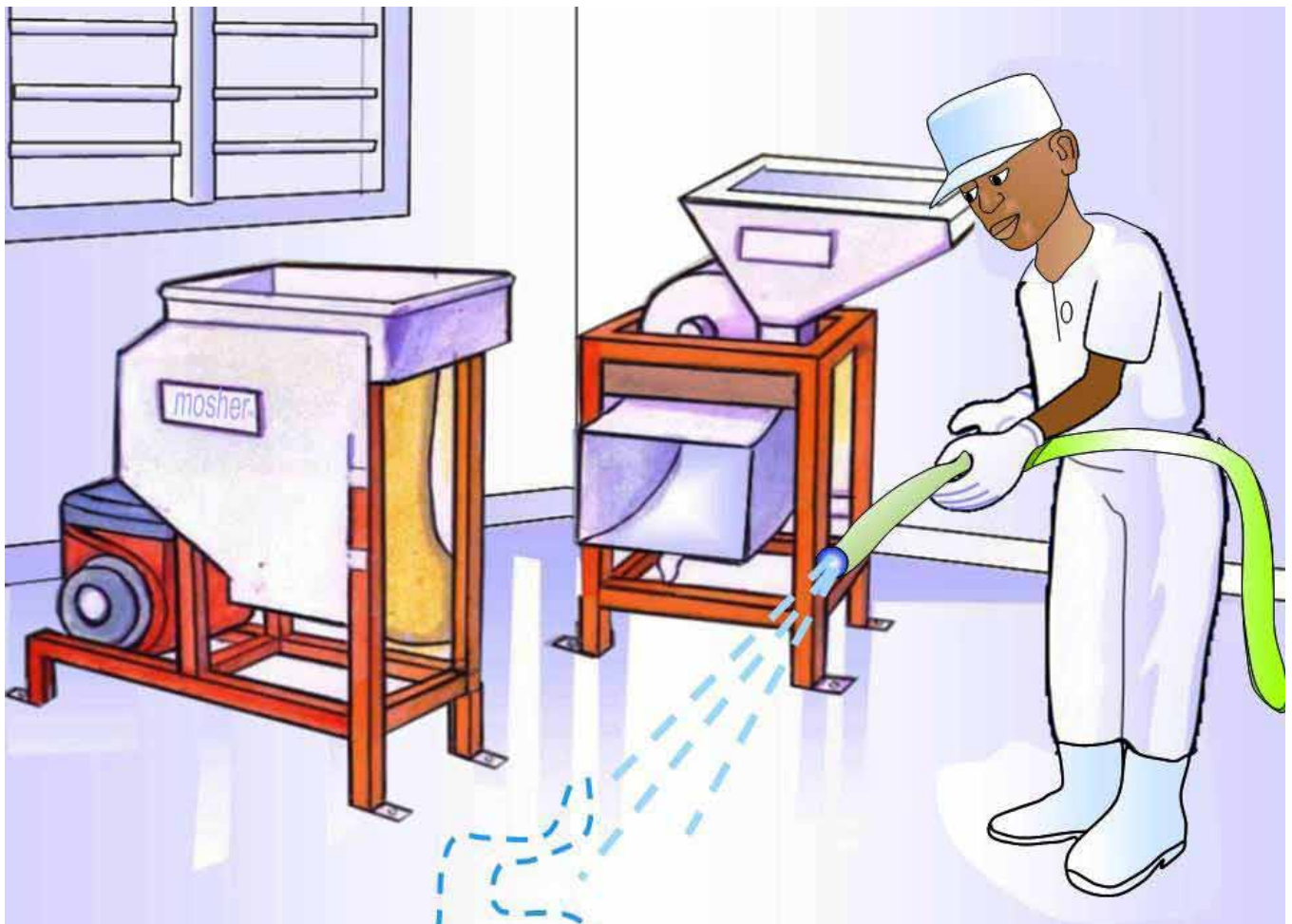
Figure 16: Clean processing floor and equipment before and after use to keep them free from dirt and dust
