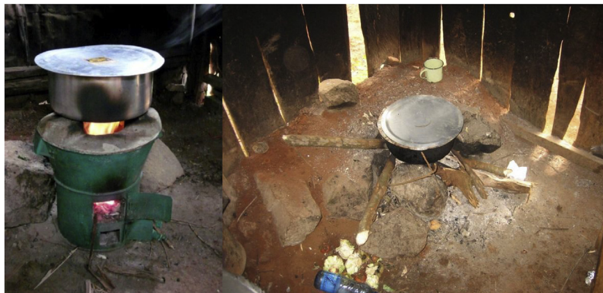
Fig. 2. Left: improved Hifadhi cooking stove and (right) traditional three-stone cooking stove used in the experiments.
