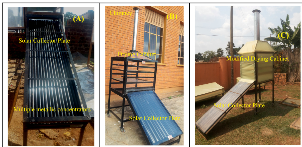
Fig. 1. Photos of an improved Hybrid Indirect Passive (HIP) dryer: where A is a modified solar collector plate consisting of multiple metallic solar collectors; B and C are the physical prototypes of the HIP without and without a non-perforated greenhouse plastic cover enclosing the dryer cabinet, respectively.
