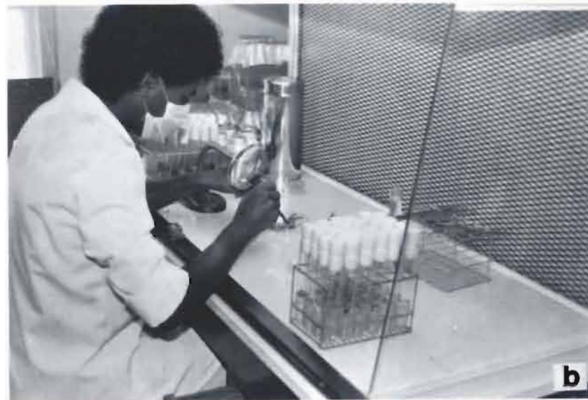
Figure 1. Preparation of the laminar air-flow cabinet for aseptic manipulations.: (a) Arrangement with stereo microscope. From left to right: sterilizing boxes containing sterile Petri dishes, light source, stereo microscope, alcohol lamp, ethanol dip with dissecting instruments on a test tube rack, medium in test tubes and glass jars; (b) arrangement with magnifier.
