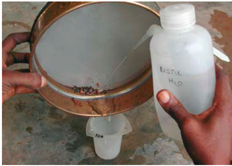
8. Using a wash-bottle, wash the debris from both the 250 and 150 \mu\text{m} sieves into beakers for collection.
