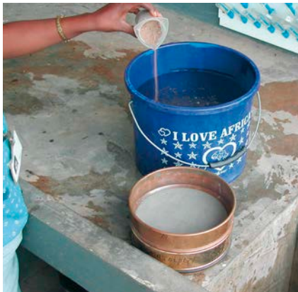
3. Pour the pre-measured dry soil sub-sample into the water.
