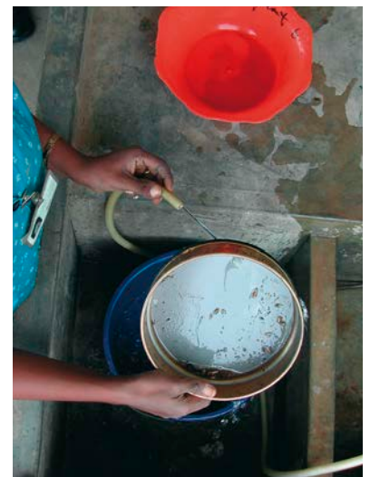
7. Rinse down each of the 2 catchment sieves, backwashing where necessary.
