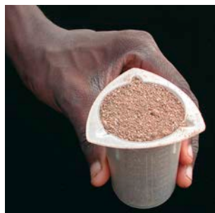
2. Measure out a standard sized sub-sample by volume, e.g. 100 ml.
