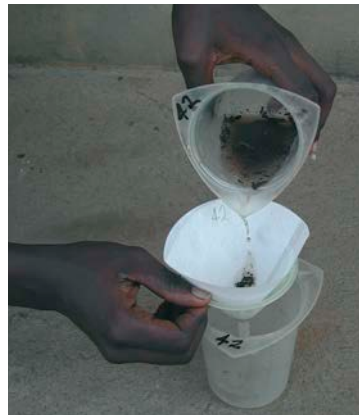
11. Pour the extraction through the filter paper.
