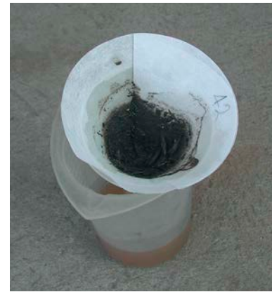
12. Leave the liquid to drain through the filter paper.
