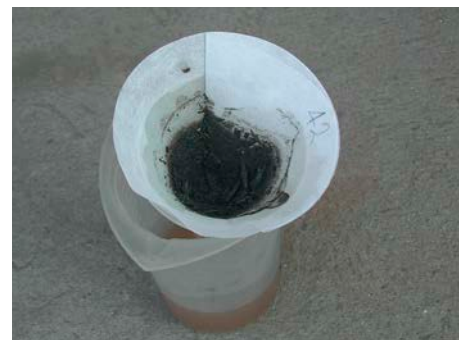
14. Leave extracts to dry in the funnel to assess cysts at a later date.
