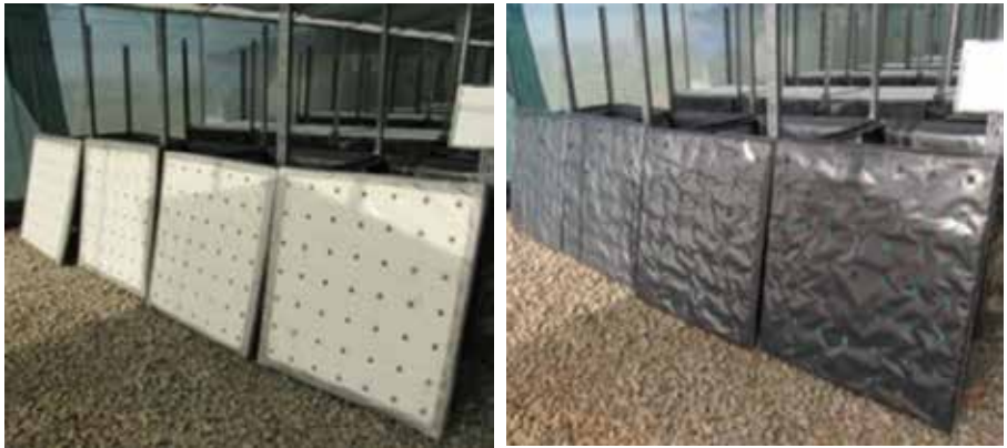
Figure 11. Perforated box' covers that serve as the upper face of tables (left) and down face in right picture.
