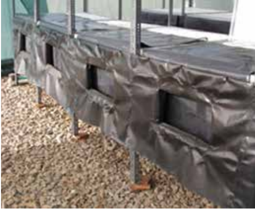
Figure 12. Styrofoam fully covered with black plastic sheet outside the box (left) and inside (right).
