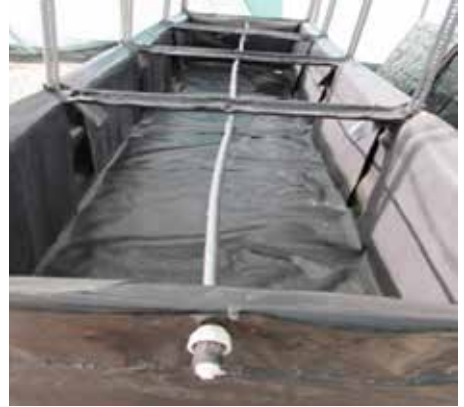
Figure 12. Styrofoam fully covered with black plastic sheet outside the box (left) and inside (right).
