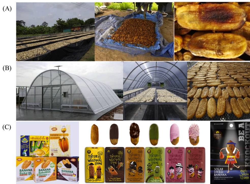
Fig. 2. Comparison of open-air sun drying and greenhouse solar drying in Thailand: (A) traditional open-air sun drying of banana in Pitsanuloke Province; (B) greenhouse dryer with parabolic shape; and (C) an example of solar-dried banana products available on the domestic and international markets.
