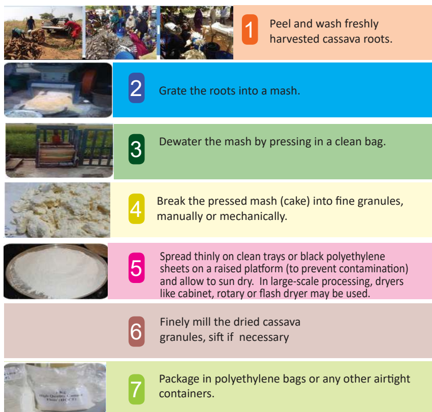
Figure 2. High quality cassava flour production process.
