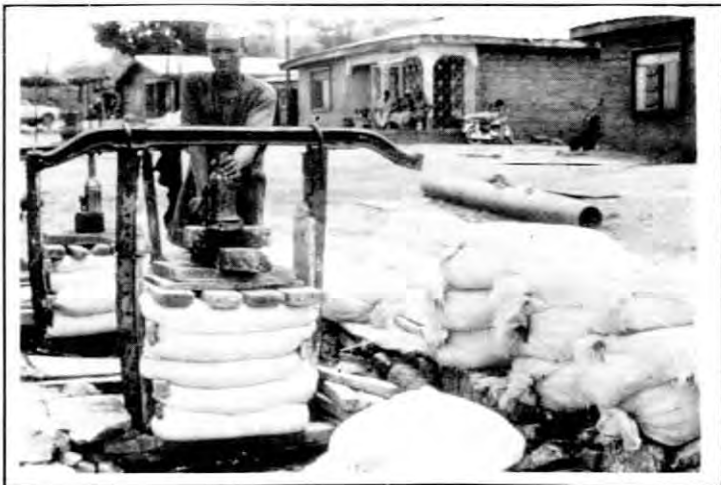
Figure 3. Grated cassava pulp sacks pressed with a hydraulic press for 2–4 days.
